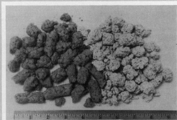
FIG. 2. Extruded dehulled soybean collets (left), same collets after solvent extraction (right).
